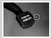
To release, firmly press the foot brake 02, then press the parking brake pedal 01 and the parking brake will release.
